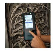
High end cable certifier up to Cat 8 and beyond for high speed cabling and data center applications
